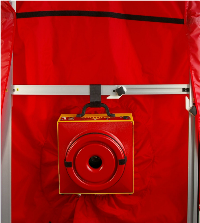
Retrotec Model Q42 consists of a DM-2, a DU-220 Fan and a cloth door panel.
