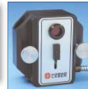
T-266 Target The S-640 features a true 4-axis target that reads both center and angle simultaneously.
